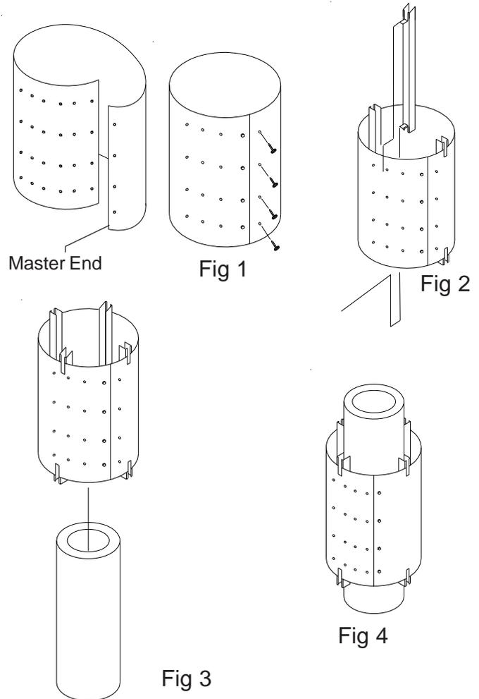
2. When properly formed, the "master" end of the panel will overlap the marked holes and the Shield will be 2" greater in diameter than the OD of the pipe. Secure in place with 4 sheet metal screws (item 4). (See Figure 1).
